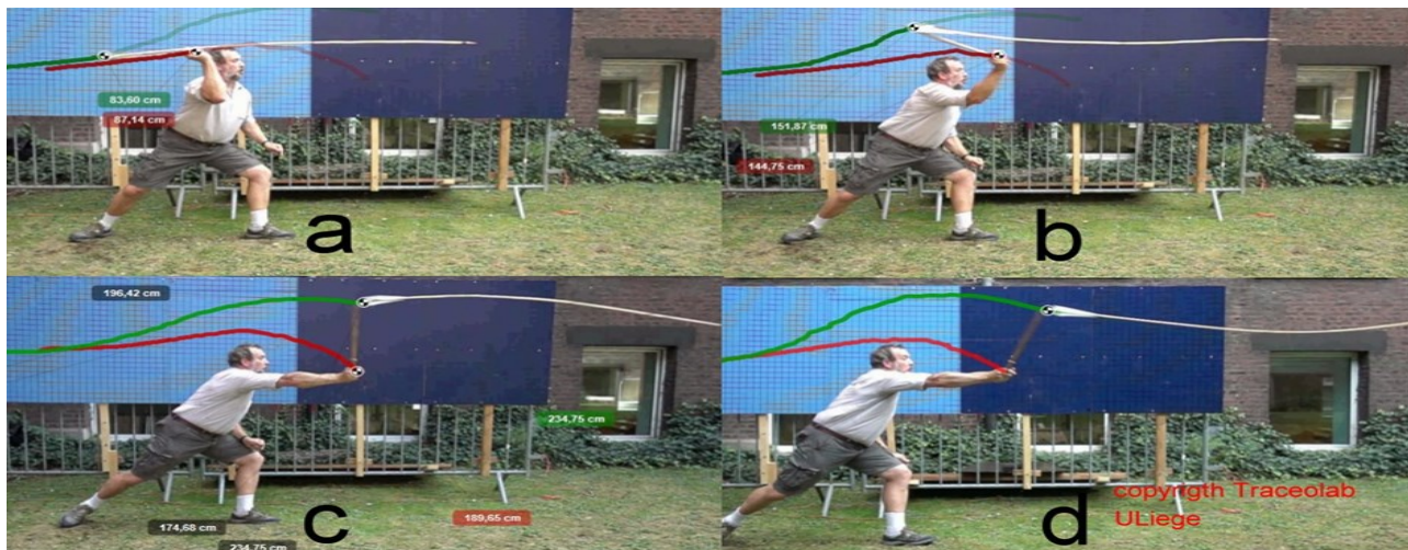
Fig. 1. The flexing of the dart during the propulsion phase. a, first convex flexing of the dart at the end of the linear phase. b, second concave flexing of the dart when the hook of the spear-thrower rises (beginning of the elliptical phase). c, Third convex bend caused by the descent of the hook at the end of the elliptical phase. d, dart too flexible at the moment of spear-thrower separation, its very high spine (14.5 cm) causes a “bend delay” (adapted from Lepers et al., 2024).
