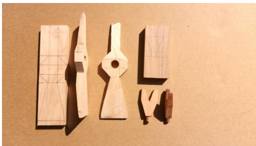
Above is example of an atlatl handle before file and sanding removes the seam where wedge shape meets donut shape.
