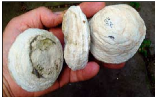
Figure 13. Three discoidal concretions of diatomite from Trenches E, F, and H. The greatest diameter of the middle specimen is 74 mm.
